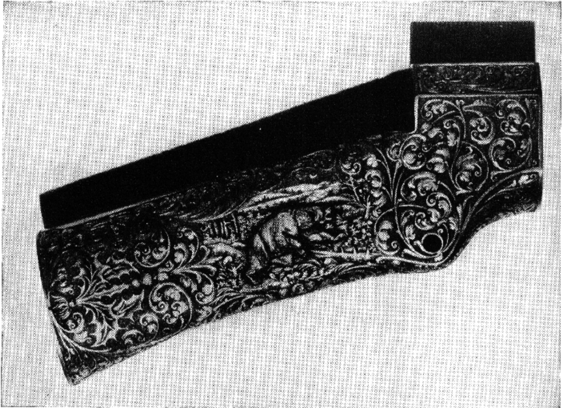
Fig. 137 Ballard action engraved in high relief. The scroll design can be used for etching
