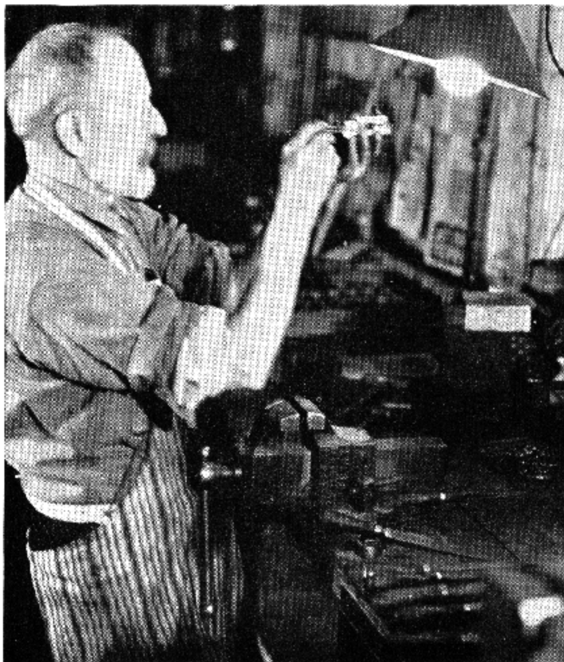
Fig. 123 Hand fitting operation on small parts as performed in the large arms plants
