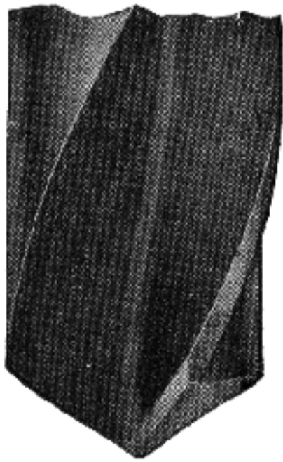
Fig. 33 Special grinding for hard metal or brass
